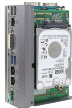
▲ POC-300 with MeziO® - R11 and 2.5" HDD
